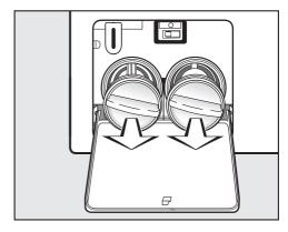
■ Remove the drain filters completely.
